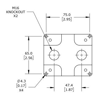
1 HOLE, 22mm, 83 X 72 X 53mm (HXWXD), WALL MOUNT, WITH KNOCKOUTS, FIBERGLASS-REINFORCED POLYCARBONATE, BLACK BODY / GRAY COVER, SCREW COVER.
