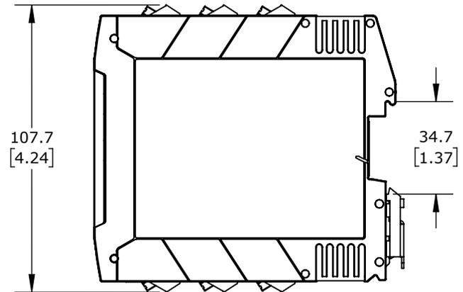
ENDRESS+HAUSER INTRINSICALLY SAFE ANALOG INPUT ISOLATOR, 0-20 MA OR 4-20 MA INPUT, (2) 0-20 MA OR (2) 4-20 MA OUTPUT, 19.2-30 VDC OPERATING VOLTAGE, SCREW TERMINALS
