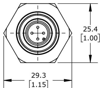
CONTRINEX RFID READ-WRITE MODULE, TUBULAR, NON-FLUSH MOUNT, HF COMMUNICATION, 13.56 MHZ, 26MM READ-WRITE DISTANCE, (1) 4-PIN M12 A-CODED PORT(S), IO-LINK CLASS A DEVICE AND SIO, 18MM DIAMETER X 63.5MM BODY, IP67.
