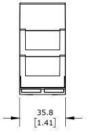
1-PHASE, 35mm DIN RAIL MOUNT, 45-135 VAC INPUT VOLTAGE, SPDT, 5A CONTACT RATING, SCREW TERMINAL(s), LED INDICATOR(s), OVERVOLTAGE, UNDERVOLTAGE AND VOLTAGE RANGE PROTECTION.
