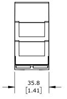
1-PHASE, 35mm DIN RAIL MOUNT, 100-300 VAC INPUT VOLTAGE, SPDT, 5A CONTACT RATING, SCREW TERMINAL(s), LED INDICATOR(s), OVERVOLTAGE, UNDERVOLTAGE AND VOLTAGE RANGE PROTECTION.
