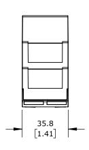
1-PHASE, 35mm DIN RAIL MOUNT, 24-130 VDC INPUT VOLTAGE, SPDT, 5A CONTACT RATING, SCREW TERMINAL(s), LED INDICATOR(s), OVERVOLTAGE, UNDERVOLTAGE AND VOLTAGE RANGE PROTECTION.
