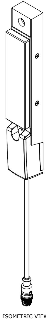
SSP SAFETY SYSTEM PRODUCTS SAFETY SWITCH, NON-CONTACT RETEACHABLE CODED RFID, MAGNETIC, 24 VDC TO LOCK, 1200N HOLDING FORCE, (2) OSSD SAFETY OUTPUT(S), PLASTIC AND ALUMINUM HOUSING, 34.4 X 239.6 X 31.1MM, (1) 8-PIN M12 QUICK-DISCONNECT, 7.8IN/200MM CABLE LENGTH.
