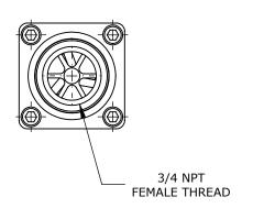
1-40 GPM, 3/4IN NPT THREAD, GLASS-FILLED NYLON.
