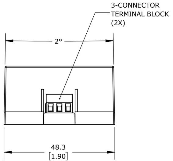
RHINO PSE-S SERIES SWITCHING POWER SUPPLY, 24 VDC @ 2.1A/50W, 120/240 VAC NOMINAL INPUT, 1-PHASE, ENCAPSULATED, PLASTIC RESIN AND FIBERGLASS HOUSING, CHASSIS MOUNT, SCREW TERMINALS.
