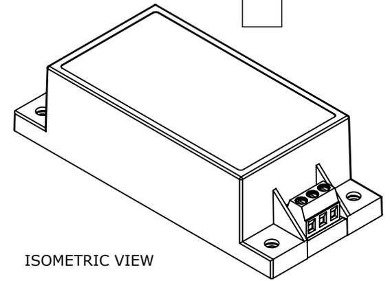
MOUNTING SCREW LOCKED TORQUE: 0.2 Nm (2 kgfcm)
