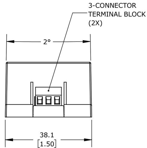
RHINO PSE-S SERIES SWITCHING POWER SUPPLY, 24 VDC @1.0A/25W, 120/240 VAC NOMINAL INPUT, 1-PHASE, ENCAPSULATED, PLASTIC RESIN AND FIBERGLASS HOUSING, CHASSIS MOUNT, SCREW TERMINALS.
