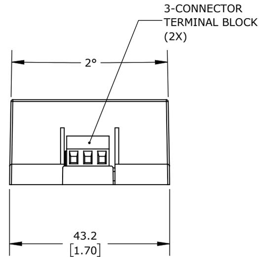
RHINO PSE-S SERIES SWITCHING POWER SUPPLY, 24 VDC @ 0.4A/10W, 120/240 VAC NOMINAL INPUT, 1-PHASE, ENCAPSULATED, PLASTIC RESIN AND FIBERGLASS HOUSING, CHASSIS MOUNT, SCREW TERMINALS.
