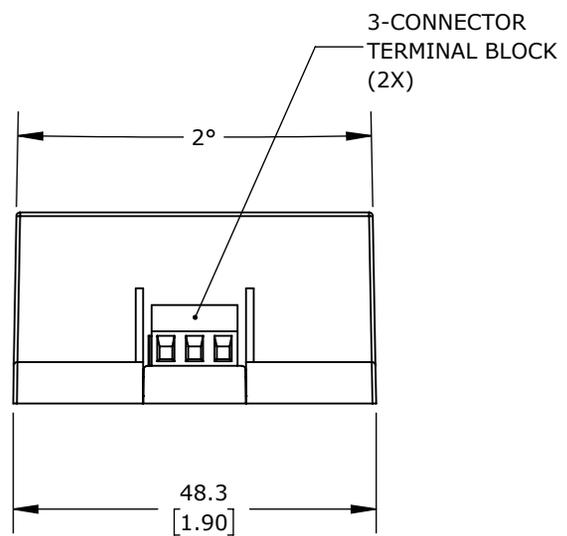
RHINO PSE-S SERIES SWITCHING POWER SUPPLY, 15 VDC @ 3.3A/50W, 120/240 VAC NOMINAL INPUT, 1-PHASE, ENCAPSULATED, PLASTIC RESIN AND FIBERGLASS HOUSING, CHASSIS MOUNT, SCREW TERMINALS.
