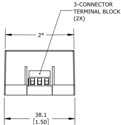
RHINO PSE-S SERIES SWITCHING POWER SUPPLY, 15 VDC @ 1.6A/25W, 120/240 VAC NOMINAL INPUT, 1-PHASE, ENCAPSULATED, PLASTIC RESIN AND FIBERGLASS HOUSING, CHASSIS MOUNT, SCREW TERMINALS.
