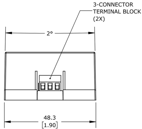
RHINO PSE-S SERIES SWITCHING POWER SUPPLY, 12 VDC @ 4.1A/50W, 120/240 VAC NOMINAL INPUT, 1-PHASE, ENCAPSULATED, PLASTIC RESIN AND FIBERGLASS HOUSING, CHASSIS MOUNT, SCREW TERMINALS.
