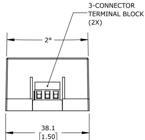
RHINO PSE-S SERIES SWITCHING POWER SUPPLY, 5.1A VDC @ 3.9A/20W, 120/240 VAC NOMINAL INPUT, 1-PHASE, ENCAPSULATED, PLASTIC RESIN AND FIBERGLASS HOUSING, CHASSIS MOUNT, SCREW TERMINALS.
