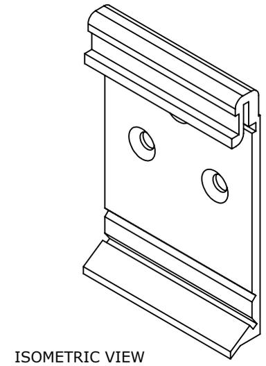
RHINO DIN RAIL MOUNTING BRACKET, ALUMINUM. FOR USE WITH 10W PSE-S SERIES ENCAPSULATED POWER SUPPLIES. MOUNTING HARDWARE INCLUDED.
