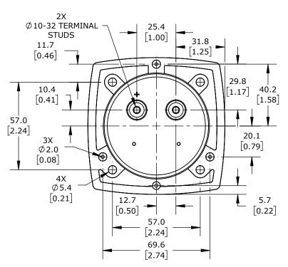
SIFAM TINSLEY SMART LOOK PANEL METER, 3.5IN ANALOG DIAL DISPLAY, 0-600 VAC, VOLTAGE INPUT, SELF CONTAINED, MOVING IRON, ROUND 3-HOLE MOUNT
