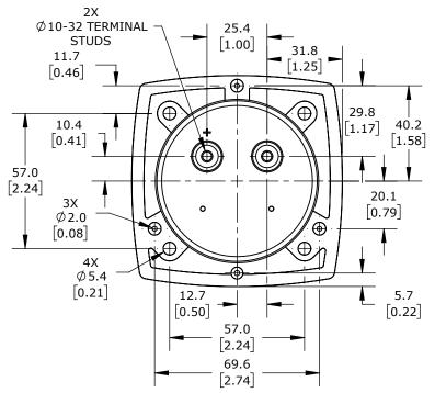
SIFAM TINSLEY SMART LOOK PANEL METER, 3.5IN ANALOG DIAL DISPLAY, 0-1000A DC, VOLTAGE INPUT, SHUNT RATED, MOVING COIL, ROUND 3-HOLE MOUNT
