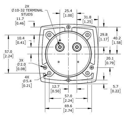
SIFAM TINSLEY SMART LOOK PANEL METER, 3.5IN ANALOG DIAL DISPLAY, 0-5A DC, CURRENT INPUT, SELF CONTAINED, MOVING COIL, ROUND 3-HOLE MOUNT
