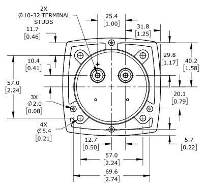
SIFAM TINSLEY SMART LOOK PANEL METER, 3.5IN ANALOG DIAL DISPLAY, 4-20MA, CURRENT INPUT, SELF CONTAINED, MOVING COIL, ROUND 3-HOLE MOUNT
