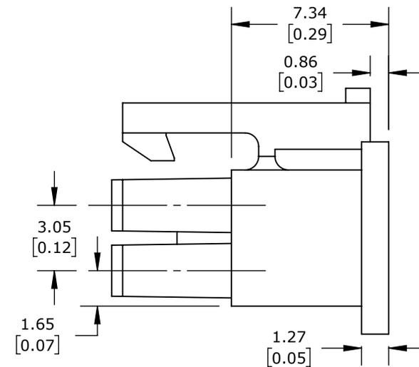
AUTOMATIONDIRECT DRIVE BRAKE CONNECTOR, REPLACEMENT, 4-PIN, FOR USE WITH ALL LS ELECTRIC PHOX SERIES DRIVES, REQUIRES PHOX-CON-D DRIVE STO/BRAKE CRIMP PINS
