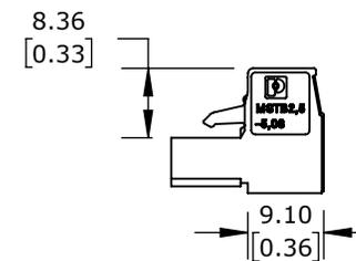
AUTOMATIONDIRECT DRIVE POWER CONNECTOR, REPLACEMENT, 8-PIN, FOR USE WITH ALL LS ELECTRIC PHOX SERIES DRIVES
