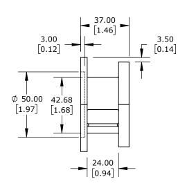
LIKA ELECTRONIC ROUND MOUNTING FLANGE, 61mm BOLT HOLE CIRCLE, METAL, FOR USE WITH LIKA ELECTRONIC AQ58 SERIES ENCODERS, MOUNTING HARDWARE INCLUDED
