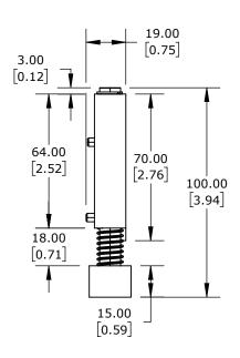
LIKA ELECTRONIC SPRING-LOADED ENCODER MOUNT, METAL. FOR USE WITH LIKA ELECTRONIC AQ58 SERIES ENCODERS, MOUNTING HARDWARE INCLUDED
