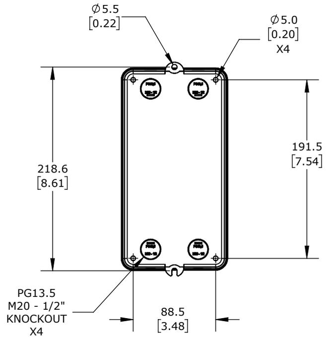
PUSHBUTTON, 25A, 2-POLE, 208-240 VAC (60Hz)/180-208 VAC (50Hz) COIL VOLTAGE, THERMAL OVERLOAD, 15.0-23.0.A ADJUSTABLE, NEMA 4/4X.
