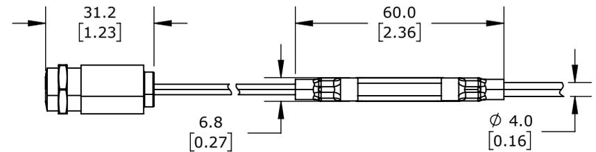
OPTRIS CSmicro LTH INFRARED PYROMETER, -50-1030 DEG C, 8-14  $\mu$ m SPECTRAL RANGE, 0-5 VDC, 0-10 VDC, ALARM OR PULSE OUTPUT, 5-30 VDC OPERATING VOLTAGE, M12x1 THREADED END MOUNT, 6m INTEGRAL 5-CONDUCTOR SHIELDED CABLE
