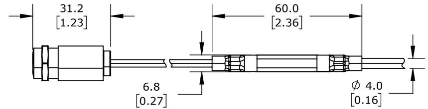
OPTRIS CSmicro 3M INFRARED PYROMETER, 50-350 DEG C, 2.3 µm SPECTRAL RANGE, 4-20mA ALARM OR PULSE OUTPUT, 5-30 VDC OPERATING VOLTAGE, M12x1 THREADED END MOUNT, 6m INTEGRAL 5-CONDUCTOR SHIELDED CABLE
