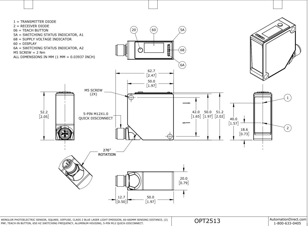
PNP, TEACH-IN BUTTON, 650 HZ SWITCHING FREQUENCY, ALUMINUM HOUSING, 5-PIN M12 QUICK-DISCONNECT. NOT TO PART DIMENSIONS MAY DIFFER SLIGHTLY 3rd
