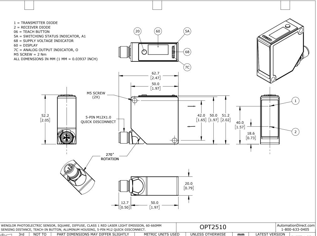
SENSING DISTANCE, TEACH-IN BUTTON, ALUMINUM HOUSING, 5-PIN M12 QUICK-DISCONNECT. 3rd NOT TO
