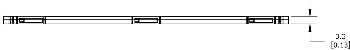
WENGLORTPL ANGLE CHANGER, LINE LIGHT, PLUS OR MINUS 9 X 16 DEGREES, POLARIZATION FILTER. FOR USE WITH M-EBAR BAR LIGHTS.
