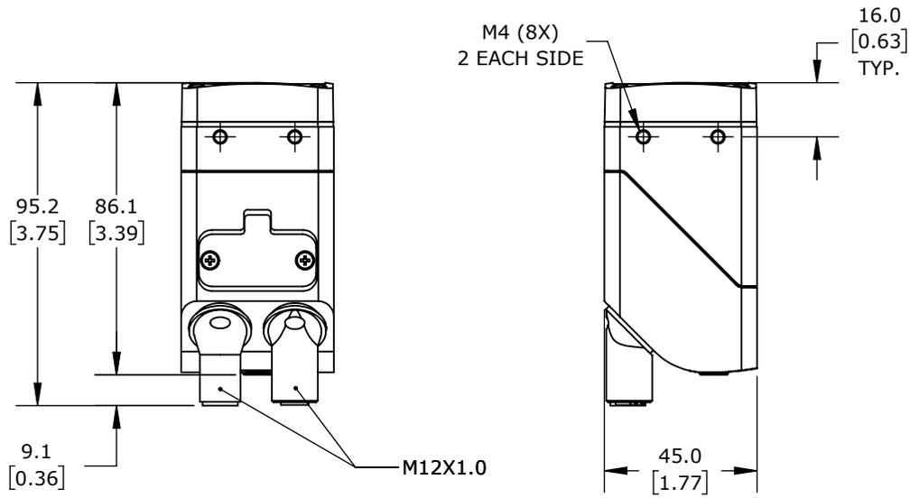
IFM EFECTOR O2I SERIES BARCODE SCANNER, INDUSTRIAL MACHINE MOUNT, 1D AND 2D, IMAGER, INFRARED LIGHT EMISSION, STANDARD LENS, 1280 X 960 OPTICAL RESOLUTION, TCP/IP AND ETHERNET/IP, IP65.
