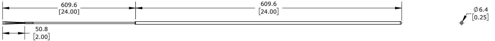
PROSENSE TEMPERATURE SENSOR, 10K-3 THERMISTOR, CUTTABLE PROBE, 24IN INSERTION LENGTH, 1/4IN PROBE DIAMETER, STAINLESS STEEL SHEATH, 24IN, 24 AWG PVC WIRE LEADS
