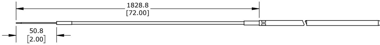
PROSENSE TEMPERATURE SENSOR, 10K-3 THERMISTOR, LEAD WIRE TRANSITION PROBE, 12IN INSERTION LENGTH, 1/4IN PROBE DIAMETER, STAINLESS STEEL SHEATH, 72IN, 24 AWG PVC AWG WIRE LEADS
