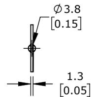
PROSENSE TEMPERATURE SENSOR, 10K-3 THERMISTOR, SPADE SENSOR, FLEXIBLE POLYIMIDE WITH ADHESIVE TAPE BACKING, 72IN, 24 AWG PVC WIRE LEADS
