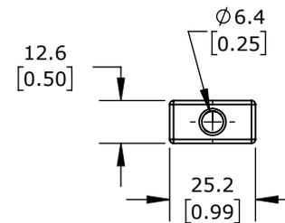
PROSENSE TEMPERATURE SENSOR, 10K-3 THERMISTOR, ATTACHED PLUG PROBE, 18IN INSERTION LENGTH, 1/4IN PROBE DIAMETER, STAINLESS STEEL SHEATH, 2-PIN STANDARD SIZE PLUG
