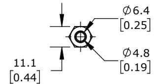
PROSENSE TEMPERATURE SENSOR, 10K-3 THERMISTOR, THREADED BOLT SENSOR, 3/8IN BOLT LENGTH, 3/16IN TIP, STAINLESS STEEL SHEATH, 1/4-28 UNF PROCESS CONNECTION, 72IN, 24 AWG PVC WIRE LEADS
