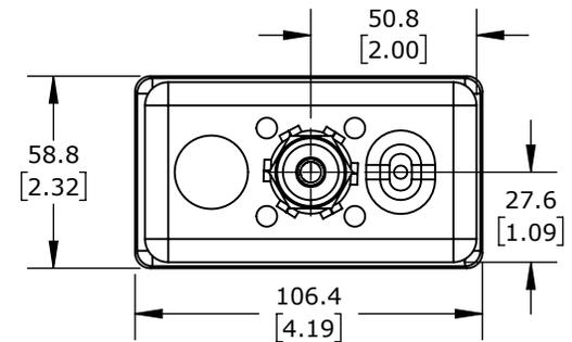
PROSENSE TEMPERATURE SENSOR, 10K-3 THERMISTOR, JUNCTION BOX PROBE, 18IN INSERTION LENGTH, 1/4IN PROBE DIAMETER, STAINLESS
