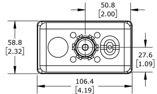
PROSENSE TEMPERATURE SENSOR, 10K-3 THERMISTOR, JUNCTION BOX SPRING-LOADED PROBE, 12IN INSERTION LENGTH, 1/4IN PROBE DIAMETER, STAINLESS STEEL SHEATH, 1/2IN MALE NPT PROCESS CONNECTION, 2IN X 4IN JUNCTION BOX WITH 24IN, 24 AWG PVC WIRE LEAD
