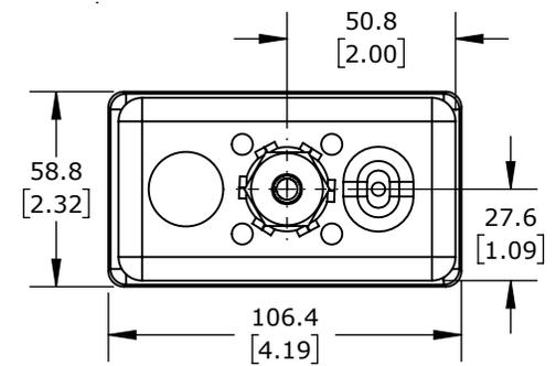
PROSENSE TEMPERATURE SENSOR, 10K-3 THERMISTOR, JUNCTION BOX PROBE, 12IN INSERTION LENGTH, 1/4IN PROBE DIAMETER, STAINLESS STEEL SHEATH, 2IN X 4IN JUNCTION BOX WITH 24IN, 24 AWG PVC WIRE LEADS
