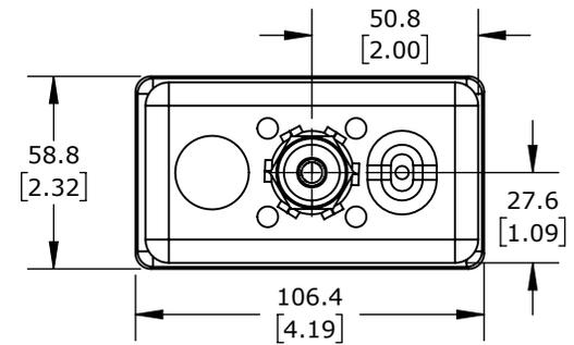
PROSENSE TEMPERATURE SENSOR, 10K-3 THERMISTOR, JUNCTION BOX PROBE, 12IN INSERTION LENGTH, 1/4IN PROBE DIAMETER, STAINLESS STEEL SHEATH, 1/2IN MALE NPT PROCESS CONNECTION, 2IN X 4IN JUNCTION BOX WITH 24IN, 24 AWG PVC WIRE LEAD
