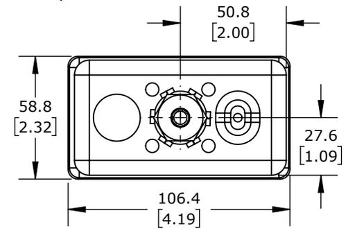
PROSENSE TEMPERATURE SENSOR, 10K-3 THERMISTOR, JUNCTION BOX PROBE, 6IN INSERTION LENGTH, 1/4IN PROBE DIAMETER, STAINLESS STEEL SHEATH, 2IN X 4IN JUNCTION BOX WITH 24IN, 24 AWG PVC WIRE LEADS
