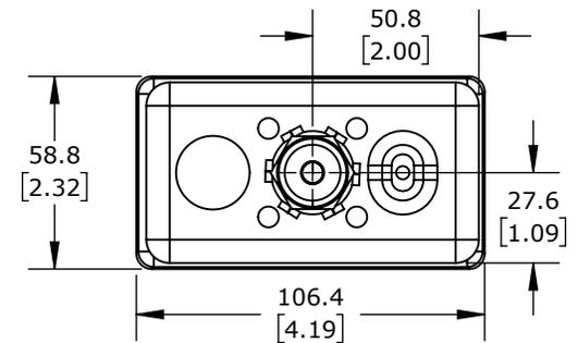
PROSENSE TEMPERATURE SENSOR, 10K-3 THERMISTOR, JUNCTION BOX SPRING-LOADED PROBE, 4IN INSERTION LENGTH, 1/4IN PROBE DIAMETER, STAINLESS STEEL SHEATH, 1/2IN MALE NPT PROCESS CONNECTION, 2IN X 4IN JUNCTION BOX WITH 24IN, 24 AWG PVC WIRE LEAD
