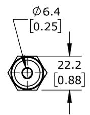
PROSENSE TEMPERATURE SENSOR, 10K-3 THERMISTOR, HEX NIPPLE SPRING-LOADED PROBE, 12IN INSERTION LENGTH, 1/4IN PROBE DIAMETER, STAINLESS STEEL SHEATH, 1/2IN MALE NPT PROCESS CONNECTION, 1/2IN MALE NPT WITH 24IN, 24 AWG PVC WIRE LEADS
