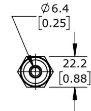
PROSENSE TEMPERATURE SENSOR, 10K-3 THERMISTOR, HEX NIPPLE PROBE, 6IN INSERTION LENGTH, 1/4IN PROBE DIAMETER, STAINLESS STEEL
