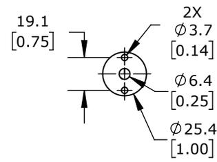
PROSENSE TEMPERATURE SENSOR, 10K-3 THERMISTOR, FLANGE MOUNT PROBE, 18IN INSERTION LENGTH, 1/4IN PROBE DIAMETER,
