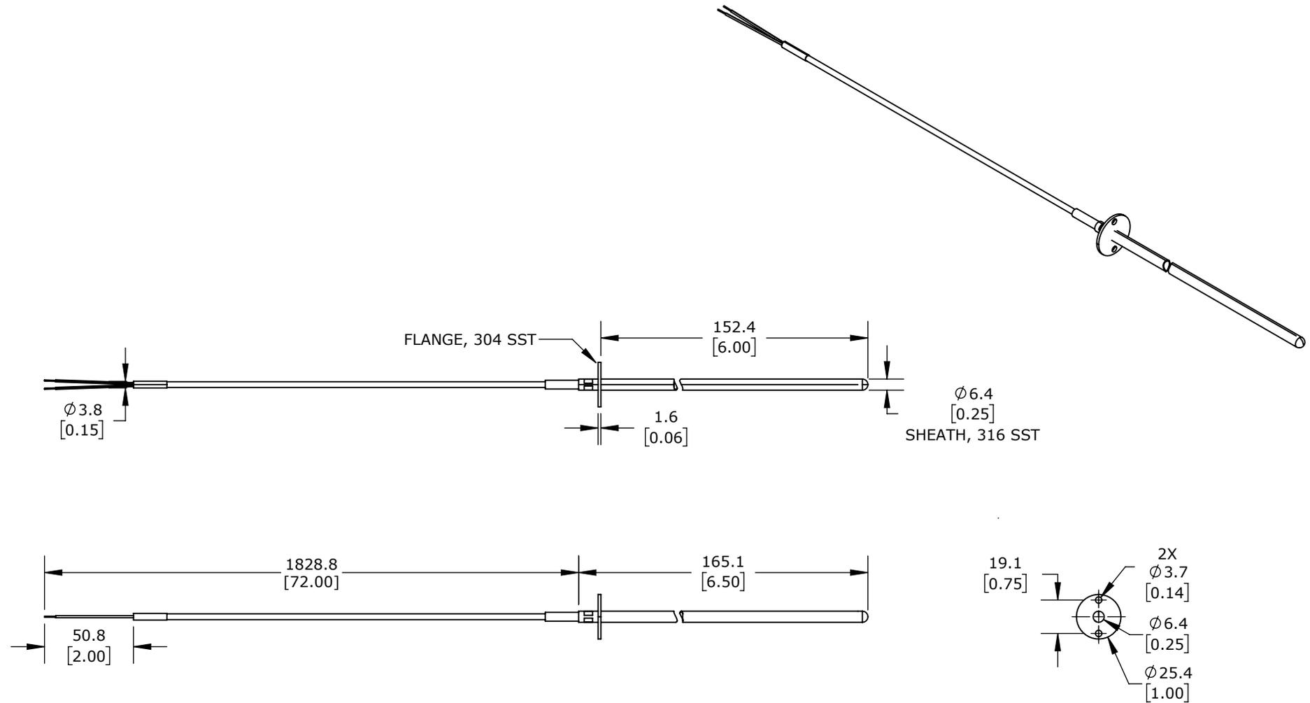
PROSENSE TEMPERATURE SENSOR, 10K-3 THERMISTOR, FLANGE MOUNT PROBE, 6IN INSERTION LENGTH, 1/4IN PROBE DIAMETER,
