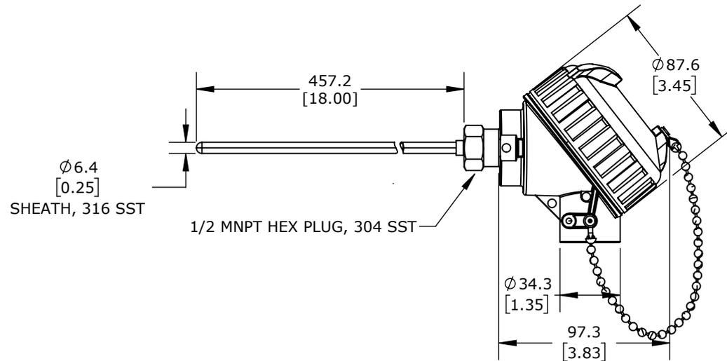
PROSENSE TEMPERATURE SENSOR, 10K-3 THERMISTOR, CONNECTION HEAD PROBE, 18IN INSERTION LENGTH, 1/4IN PROBE DIAMETER, STAINLESS STEEL SHEATH, ALUMINUM SCREW COVER HEAD WITH 24IN, 24 AWG PVC WIRE LEADS
