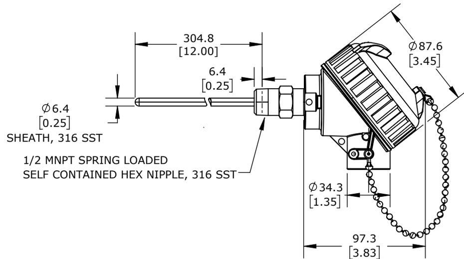
ProSense temperature sensor, 10K-3 thermistor, connection head spring-loaded probe, 12in insertion length, 1/4in probe diameter, stainless steel sheath, 1/2in male NPT process connection, aluminum screw cover head with 24in, 24 AWG PVC wire leads
