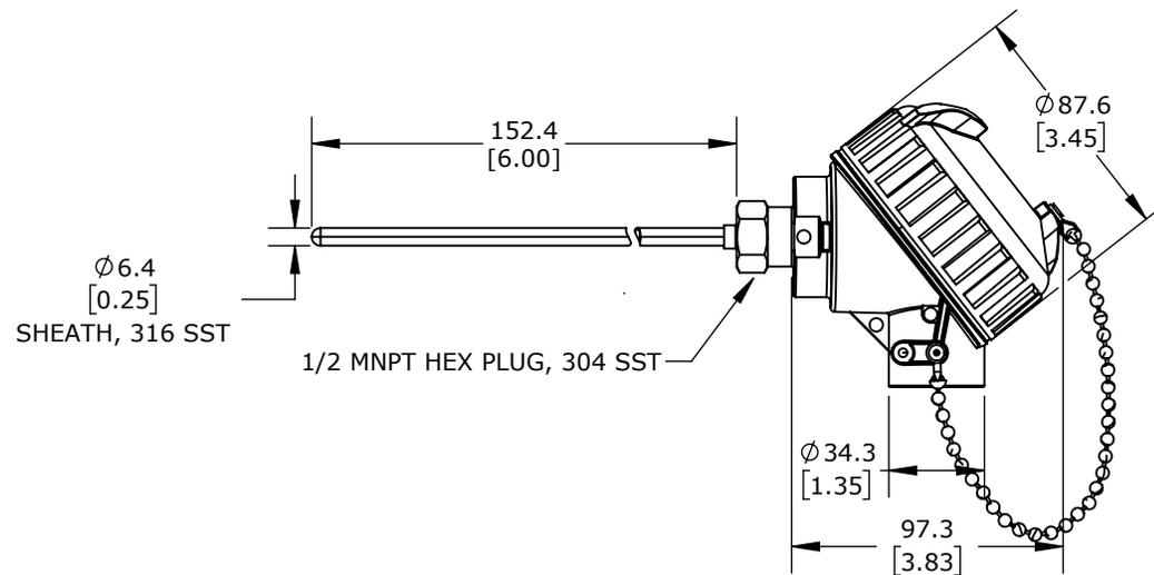
PROSENSE TEMPERATURE SENSOR, 10K-3 THERMISTOR, CONNECTION HEAD PROBE, 6IN INSERTION LENGTH, 1/4IN PROBE DIAMETER, STAINLESS STEEL SHEATH, ALUMINUM SCREW COVER HEAD WITH 24IN, 24 AWG PVC WIRE LEADS
