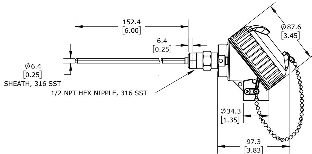
PROSENSE TEMPERATURE SENSOR, 10K-3 THERMISTOR, CONNECTION HEAD PROBE, 6IN INSERTION LENGTH, 1/4IN PROBE DIAMETER, STAINLESS STEEL SHEATH, 1/2IN MALE NPT PROCESS CONNECTION, ALUMINUM SCREW COVER HEAD WITH 24IN, 24 AWG PVC WIRE LEADS
